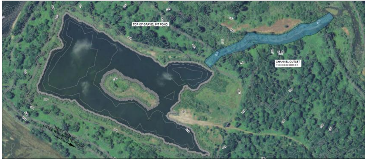
Figure 5-1. An aerial image of the BRSP gravel pond with the Alternative 1 – Channel Outlet highlighted. Alternative 1 includes excavating a connector channel between the gravel pond and Coon Creek.
