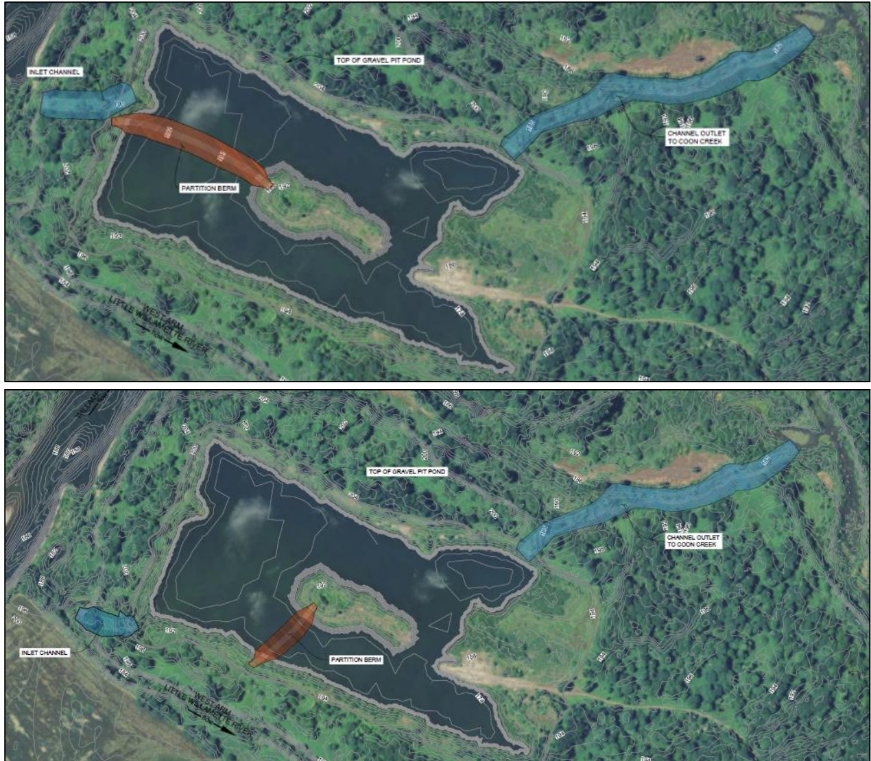
Figure 5-2. An aerial image of the BRSP gravel pond with Alternative 2A (top) and Alternative 2B (bottom) highlighted. Alternative 2 includes excavating inlet and outlet connector channels and an interior partition berm to reduce the effective flow-through area to promote native fish habitat. The sub-alternatives vary according to the inlet channel and partition berm locations.
