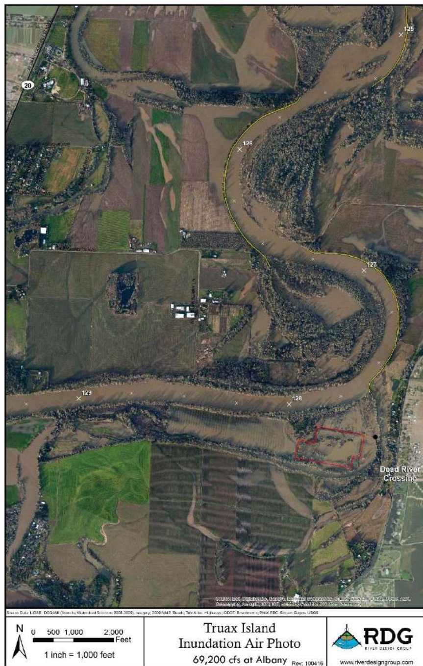
Figure 3-4. Aerial photograph of the Truax Island area taken on January 28, 2012. The USGS Albany gage registered approximately 69,200 cfs during air photo acquisition. USACE revetments are noted by the yellow lines. The Truax Island gravel pit boundary is noted by the red outline.
