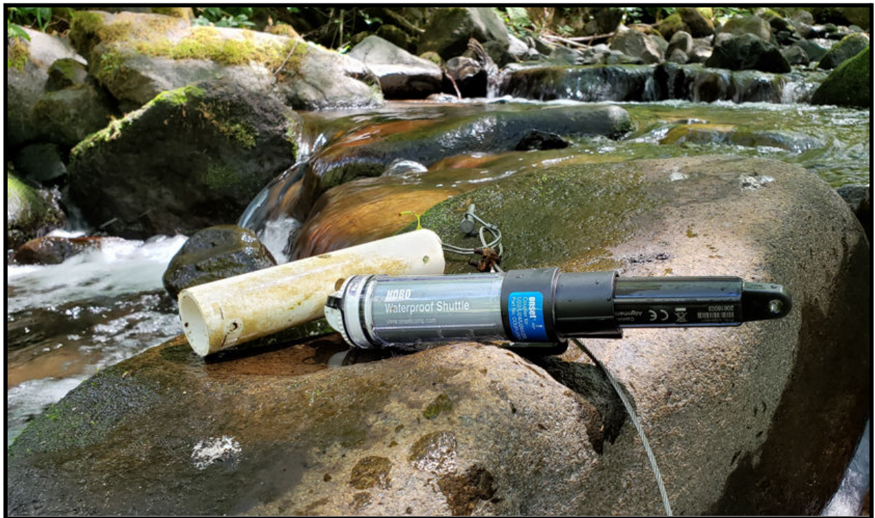
Image 4.0: Example of HOBO temperature sensor being downloaded (2019)
